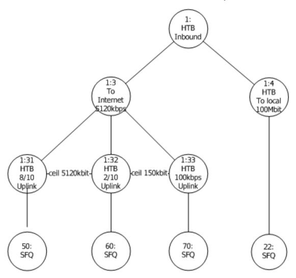
The first step in shaping the outgoing traffic is to get the ifb0 Intermediate Functional Block device (http://lartc.org/howto/index.html)" working. It turned out that the module does not load automatically, but I rather loaded it in the rc.traffic\_shaping script by:
